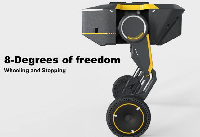
The Tita robot is a wheeled bipedal robot with perception, cognition and decision-making capabilities. Tita improves upon Direct Drive's previous robots; increasing it's degrees of freedom from 6 to 8, this means that Tita can both wheel around or walk. The smooth all-in-one shape and strong customisation makes Tita highly adaptable.
