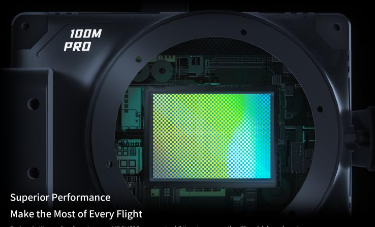
Equipped with a medium format sensor of  $43.8 \times 32.9$ mm, covering 1.7 times larger range than 35mm full-frame format. Images collected keeps a high level of color fidelity and reveal more details in highlights and shadows.
